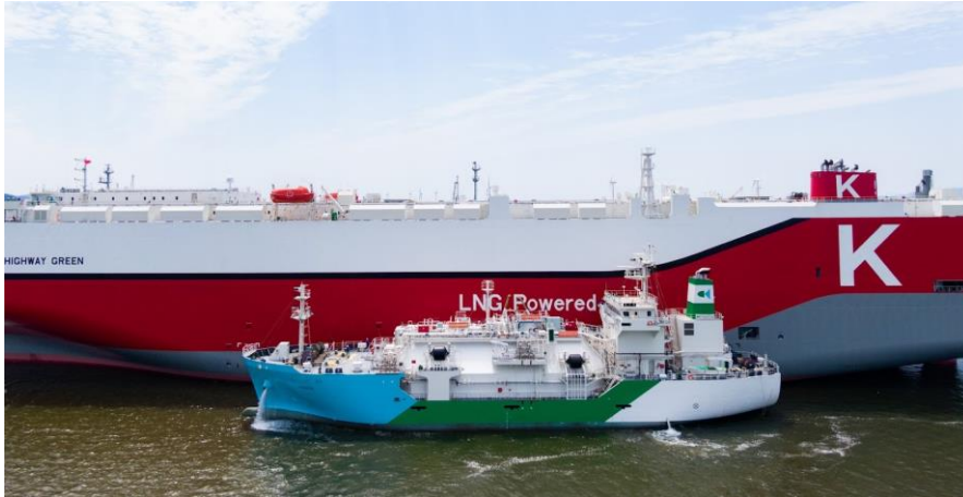
LNG bunkering vessel "KAGUYA" with a capacity of 3,500 m 3
